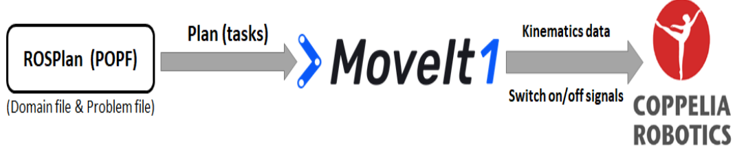
Figure 5.3: The robotic simulator framework for converting AI plan tasks to robotic numerical motion control commands and 3D printing operations.
